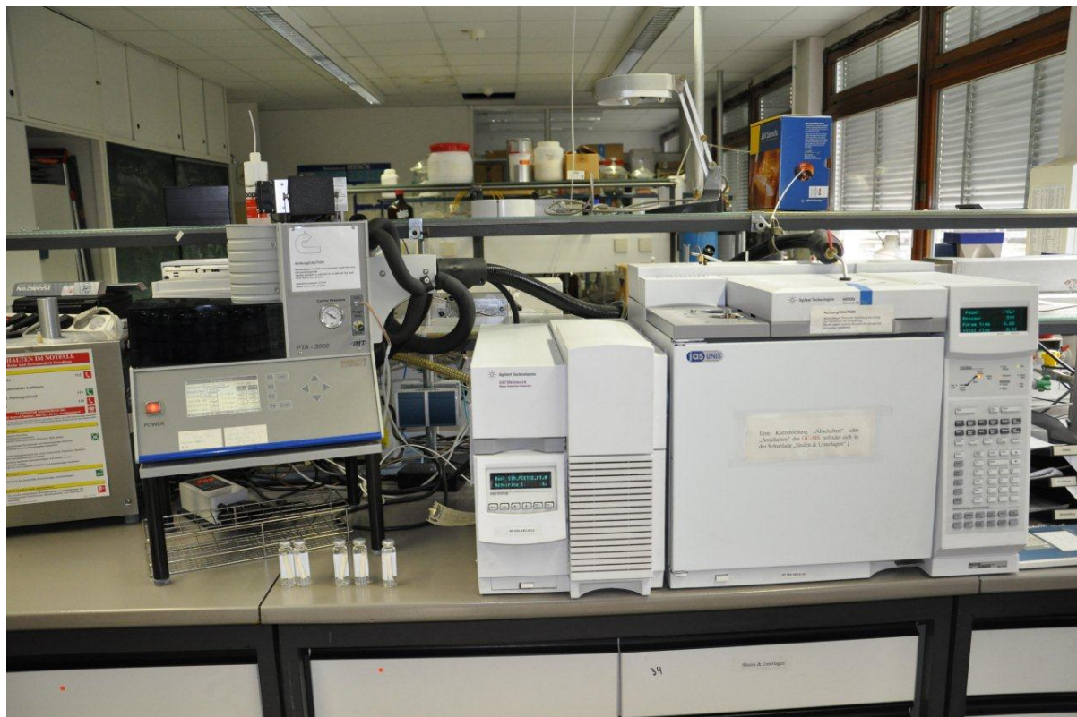
Fig. 7: Purge and Trap (left) coupled to GC-MS (right) via heated transfer lines.
