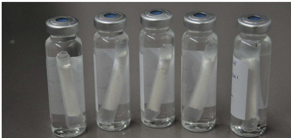
Fig. 6: Passive sampling devices stored in water in sealed headspace glas vials for storage and shipping.
